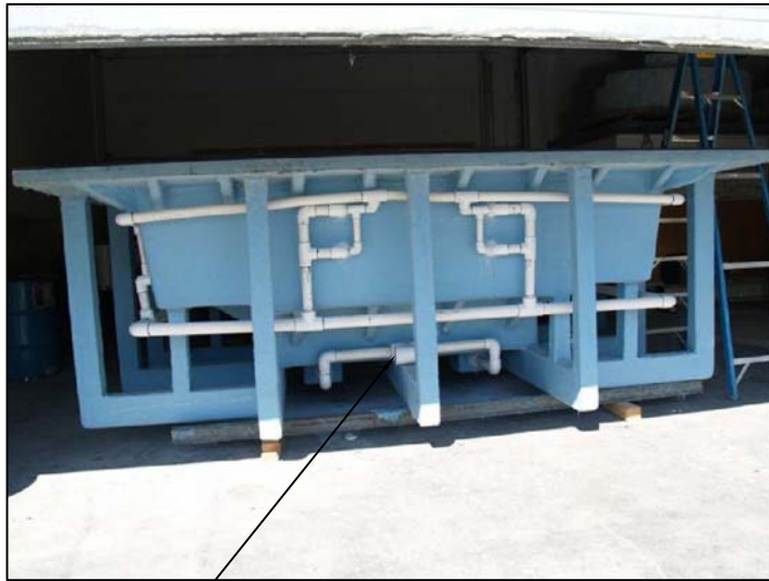
3" MAIN DRAIN SUCTION
