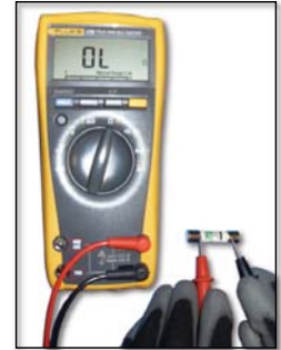
A FUSE WITH THE METER READING "BAD"
