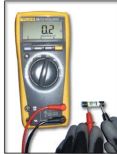
A FUSE WITH THE METER READING "GOOD"
