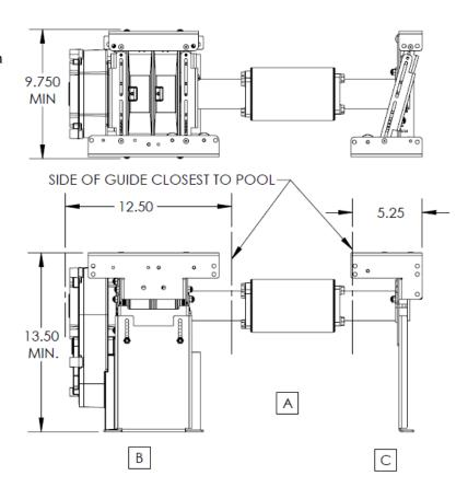
\*All dimensions on length are from the side of the guide closest to the pool Additional room recommended for ease of access.
